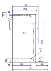
Electrical inlet (power) ΕI Refrigerant Outlet RO
